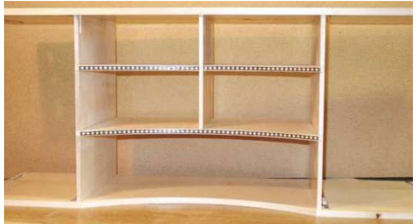
▲ Pic.16 The sycamore carcass is decorated with ebony and sycamore banding
